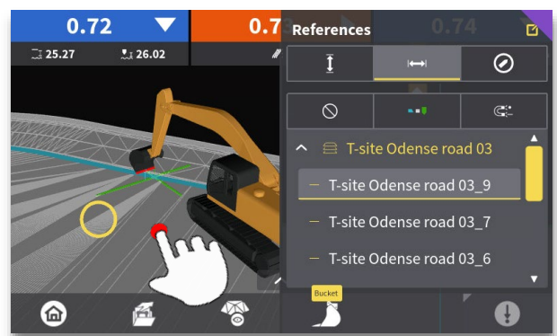
Step 4: Tap anywhere in the plan view to exit the "References" menu.
