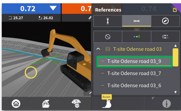
Step 3: Select desired line reference. The line closest to selected point is listed at the top.
